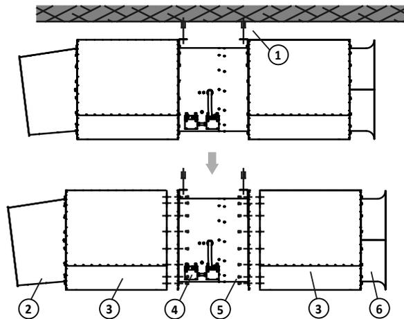
1. Certified high temperature bolts    2. Outlet nozzle    3. Silencers    4. Terminal box    5. Set screws    6. Inlet cone
