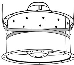
Figure 2. Lift of fan with two straps
