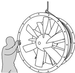
Figure 1. Lift of fan with one strap
