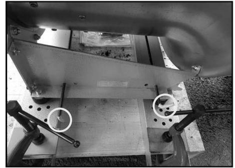
**Figure 3.** Transport rods in AZL support frame
