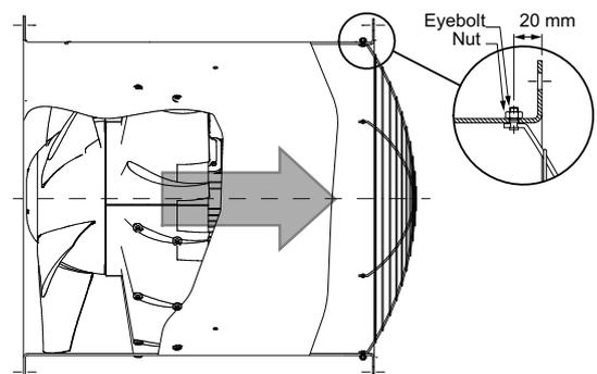
Figure 6. In-pipe installation of wire guard
