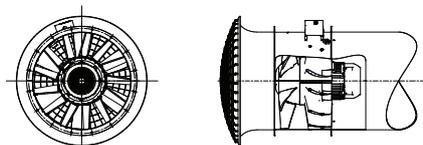
**Figure 9.** Installation in duct
