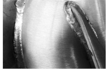
Figure 11. Impeller weldings
