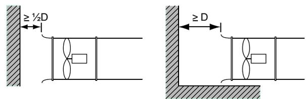
**Figure 7.** Installation spaces in ducts – optimal (left) and reduced
