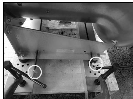
Figure 3. Transport rods in AZL support frame
