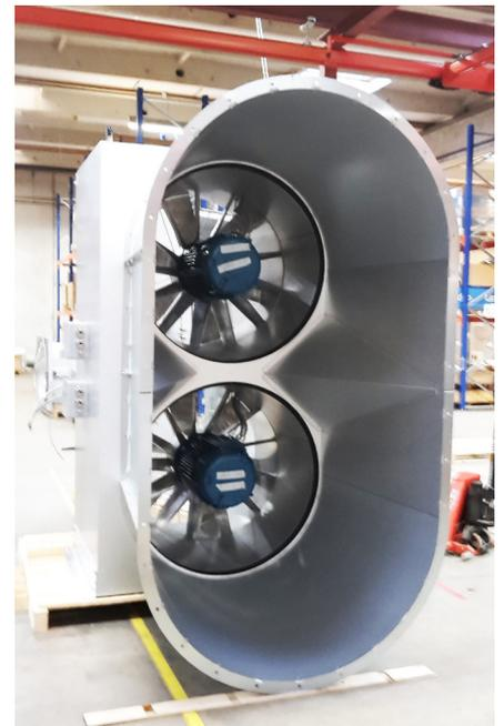
Fan array with double-diffuser
