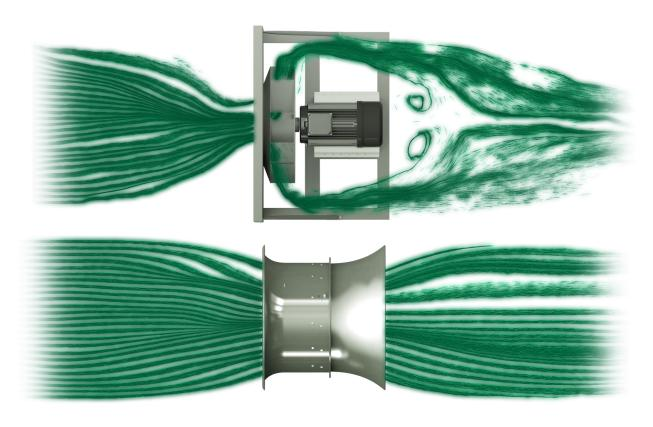
Difference in air flow between centrifugal fans and ZerAx® axial fans
