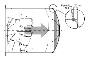
Figure 6. In-pipe installation of wire guard
