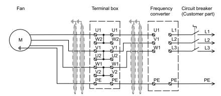
Figure 18. Frequency converter connection for all motors
