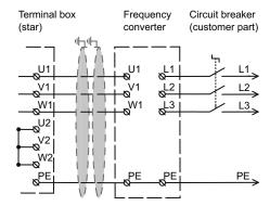
Figure 17. Terminal box star-connection
