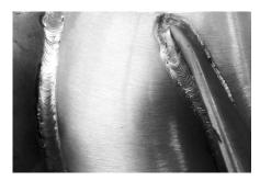
Figure 11.Impeller weldings
