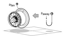
Figure 10. Measurement of pressure difference
