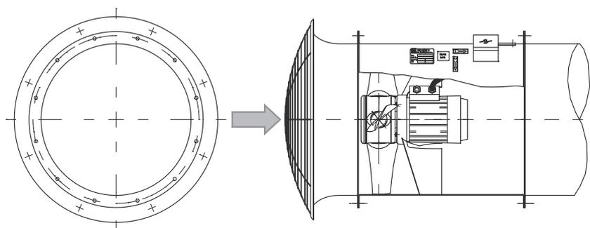
Figure 6. Inlet cone for connection to duct
