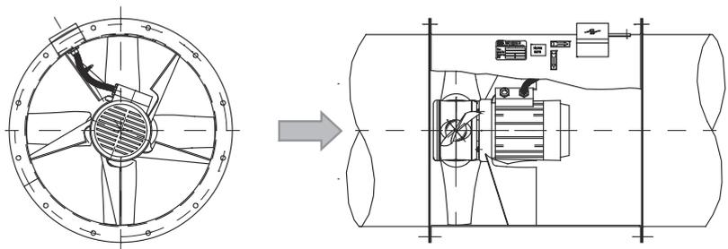
Figure 5. Installation in duct system
