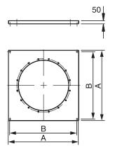
Vertical mounting plate for fan sizes Ø250 - Ø500
