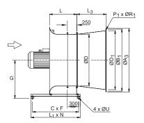
Support frame for ACG with short diffuser - hub sizes Ø403 and Ø578
