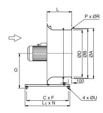
Support frame for ACG hub sizes Ø403 and Ø578
