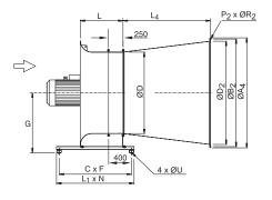
Support frame for ACG with long diffuser - hub sizes Ø403 and Ø578
