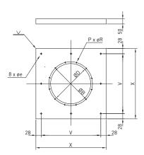
Vertical mounting plate for fan sizes Ø560 - Ø2000
