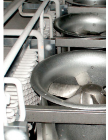
ZerAx® fans installed in freeze tower and operating at minus 30 °C
