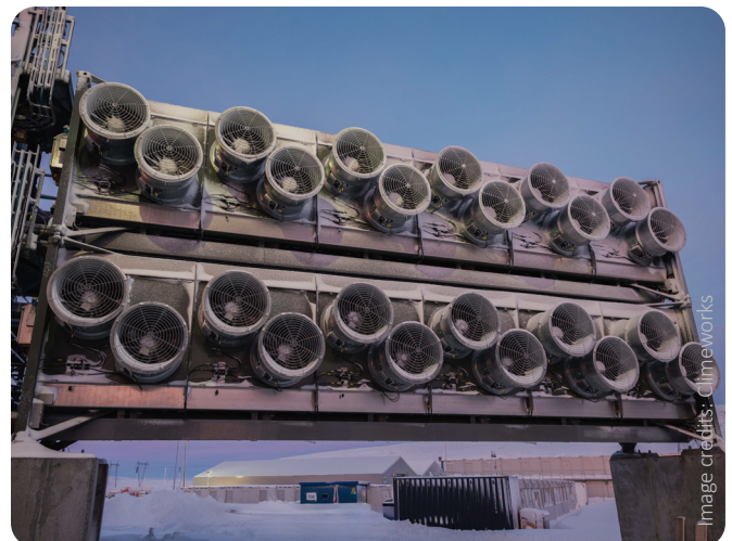
Two CO 2 collector containers, each equipped with 12 ZerAx fans
